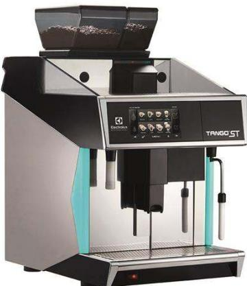
**604043 (ST121CE40052K)** Full-automatic machine, 1 group, 270x40 ml espresso cup/hr, 6,5 liter steam/coffee boiler, 1x1,7 kg and 1x1,2 kg coffee hopper, programmable water and steam, 1xTango Cappuccinatore device with double function L: for hot milk and C: for foam by air injection
